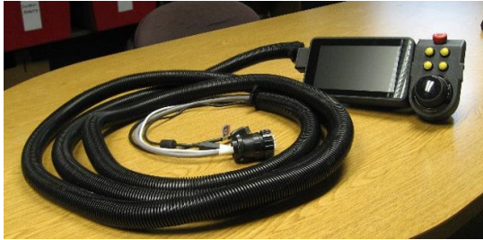
Fig. 4: Open-Source Teach Pendant Prototype [17]
